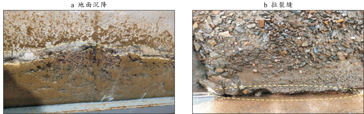
图 3 坡体变形过程中的沉降和拉裂缝 Fig.3 Subsidence and tension cracks during slope deformation
