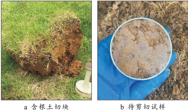
图 2 直剪试验取样图解 Fig.2 Sampling diagram for straight shear test
